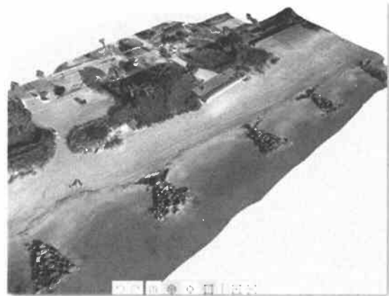
3d model created from photos captured with CB&I's Inspire 1 drone using in-house photogrammetry software.
