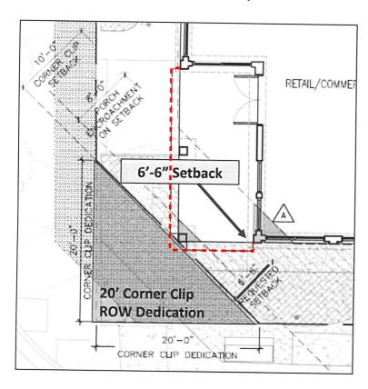
First Floor concrete overhang was built slightly different from what was approved, as the corner wraps around the corner and intrudes in the Corner Clip ROW Dedication.
