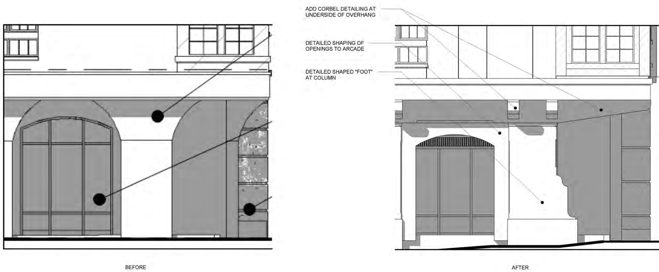
3 BUILDING III ARCADE EDGE AT WEST END 1/4" = 1'-0"
