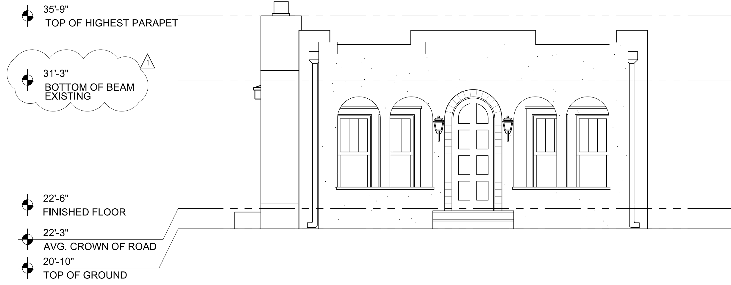
4 WEST ELEVATION-EXISTING SCALE: 1/4"=1'-0"
