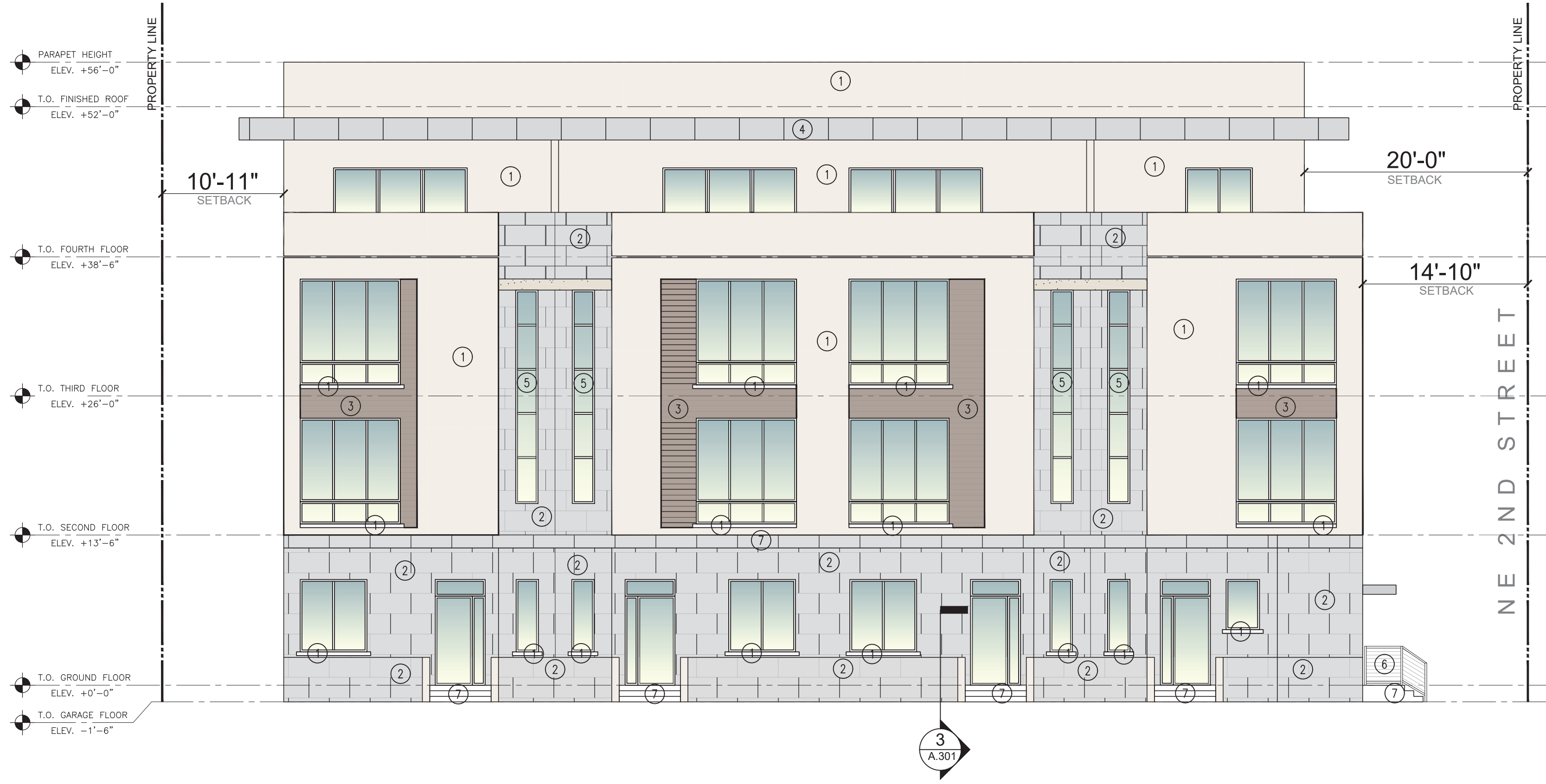
1 WEST ELEVATION A.201 BUILDING 1
