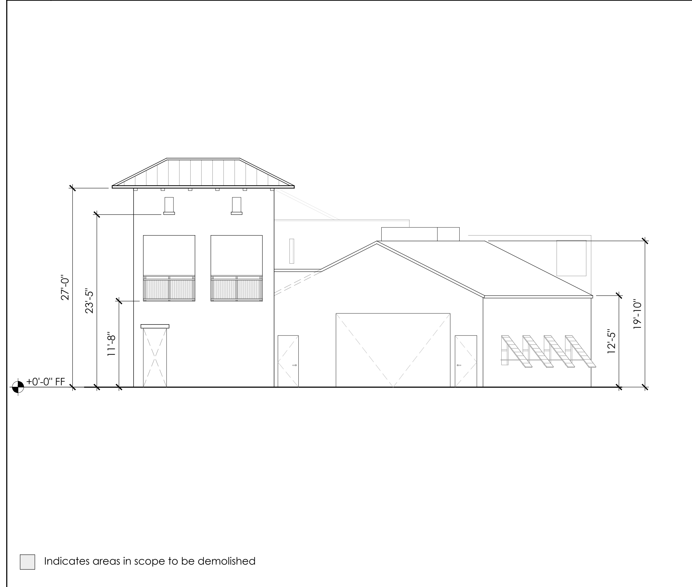
3 Demolition South Exterior Elevation 1/8" = 1'-0"
