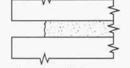
Fig. 1. Properly prepared joint.
