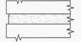
Fig. 2. Improperly prepared joint — too shallow.
