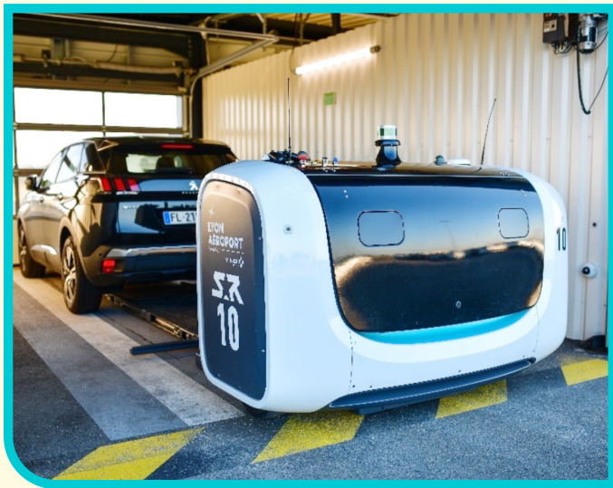
Image 34: Example of robotic valet (Stanley Robotics)
