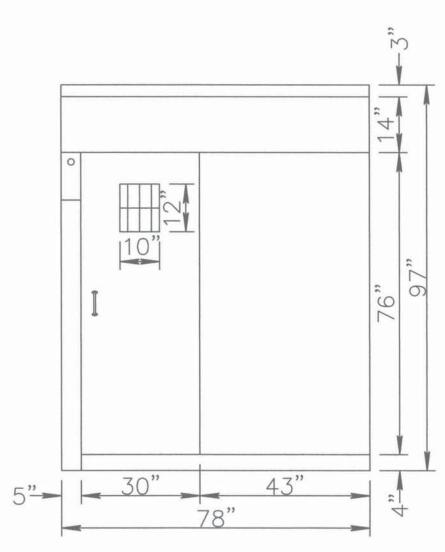
NOTE: WINDOW HAS A HINGED DOOR OVER IT. HINGE IS AT THE TOP OF THE DOOR WITH A SELF LOCKING MANUAL HARDWARE.
