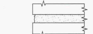
Fig. 2. Improperly prepared joint — too shallow.
