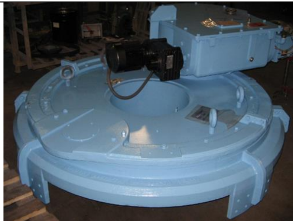
Dorr-Oliver® Drive Rebuild
