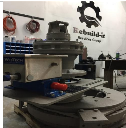
WesTech Drive Rebuild
