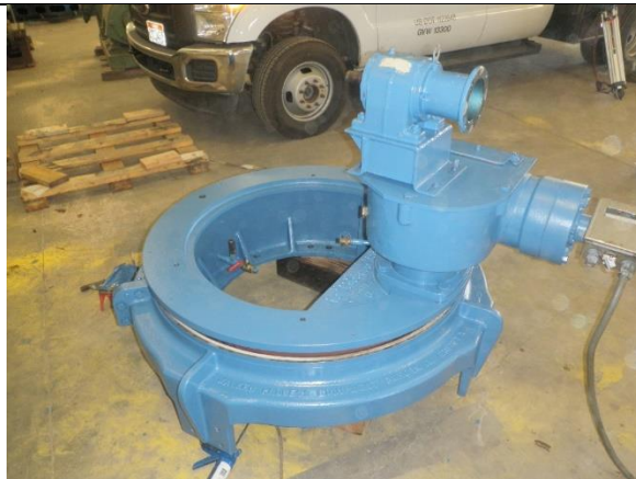
Walker Drive Rebuild
