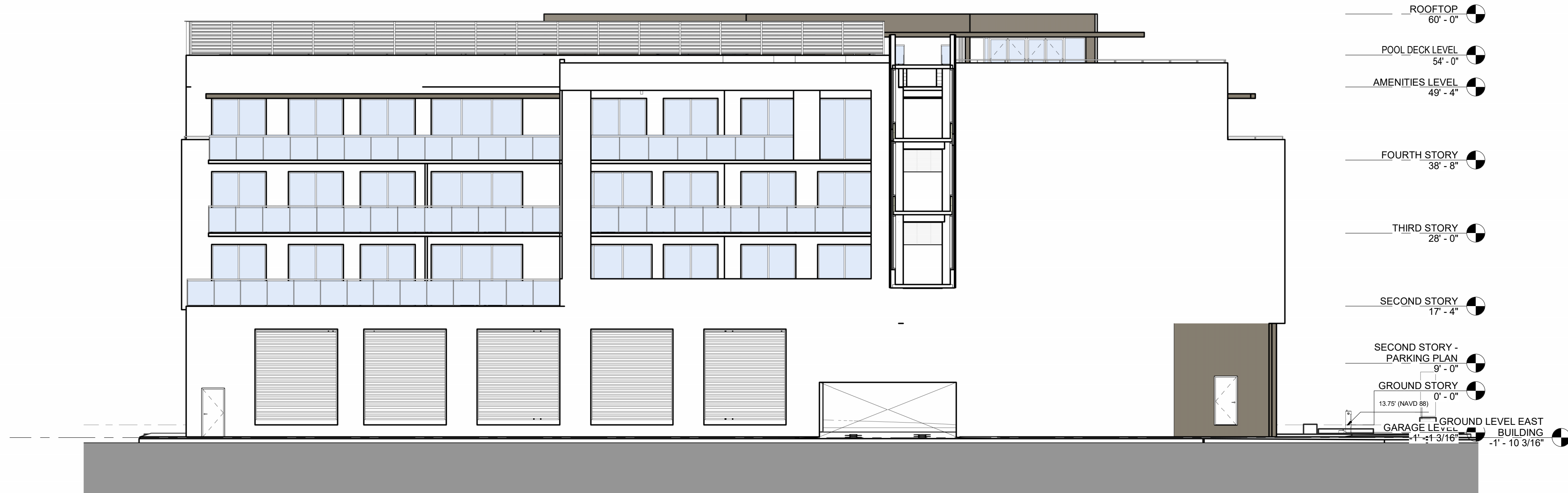
1 EAST ELEVATION (DRIVEWAY) A203.1 SCALE: 3/32" = 1'-0"
