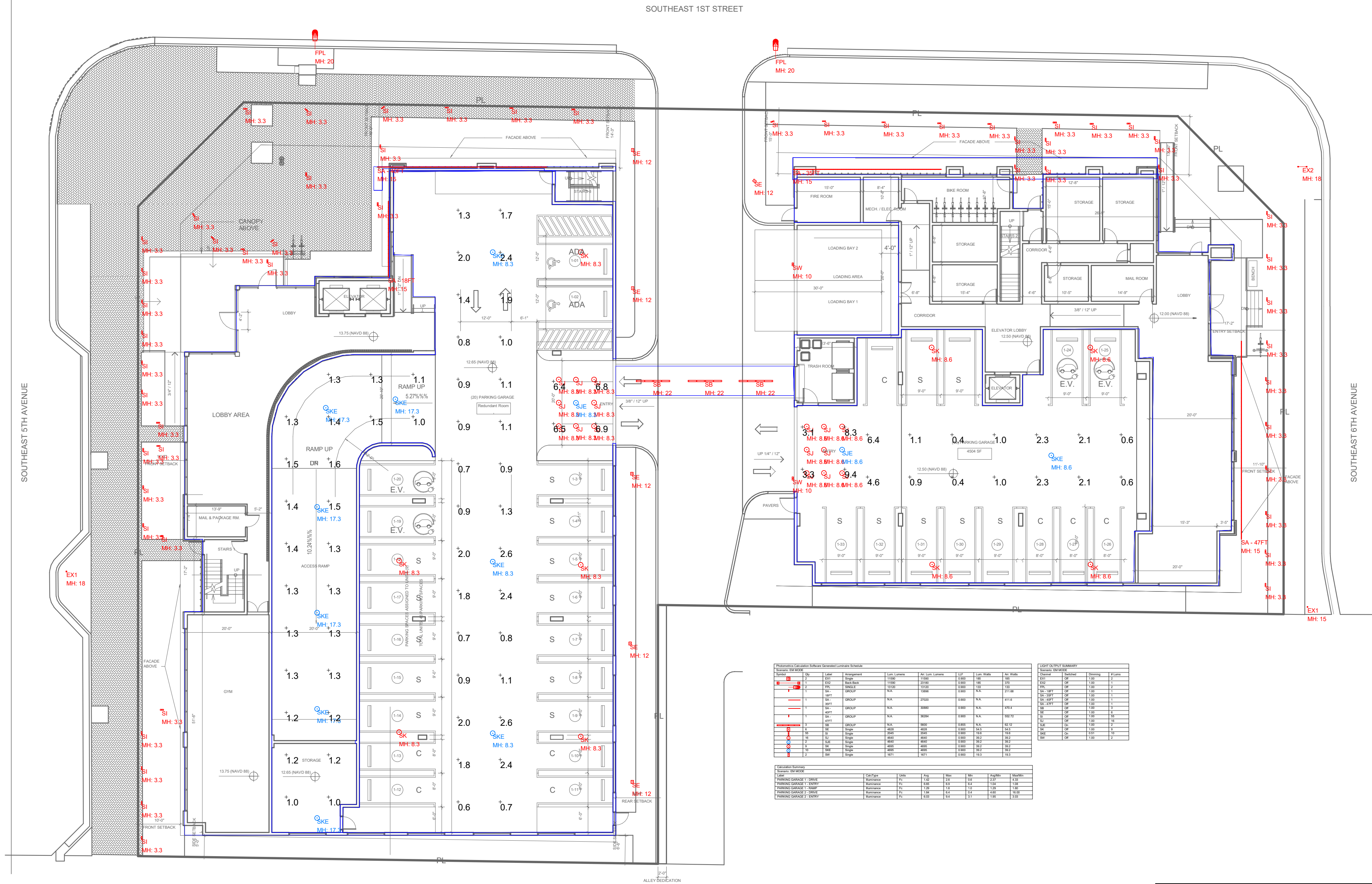
GROUND LEVEL - PHOTOMETRICS EMERGENCY PLAN 1/16" = 1'-0"
