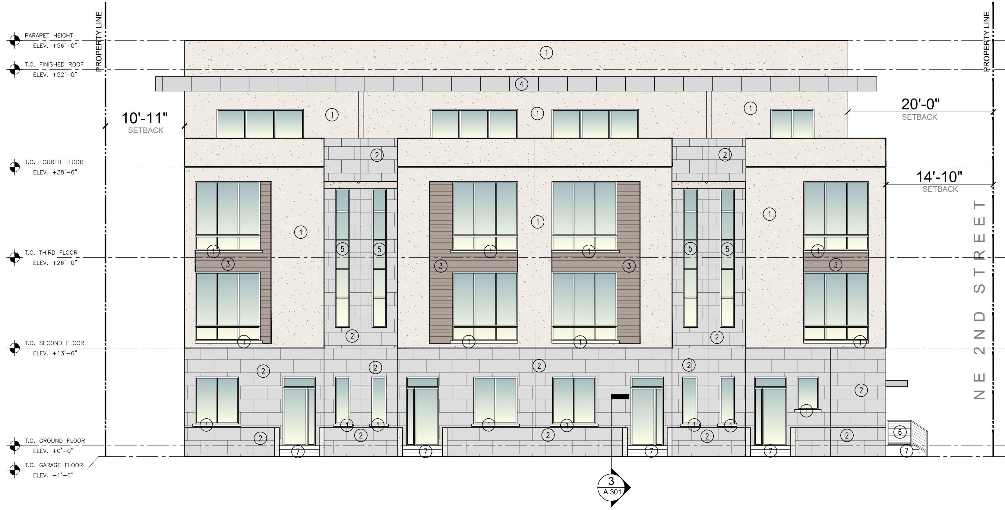
1 A.201 BUILDING 1 WEST ELEVATION SCALE: 1/8" = 1'-0"
