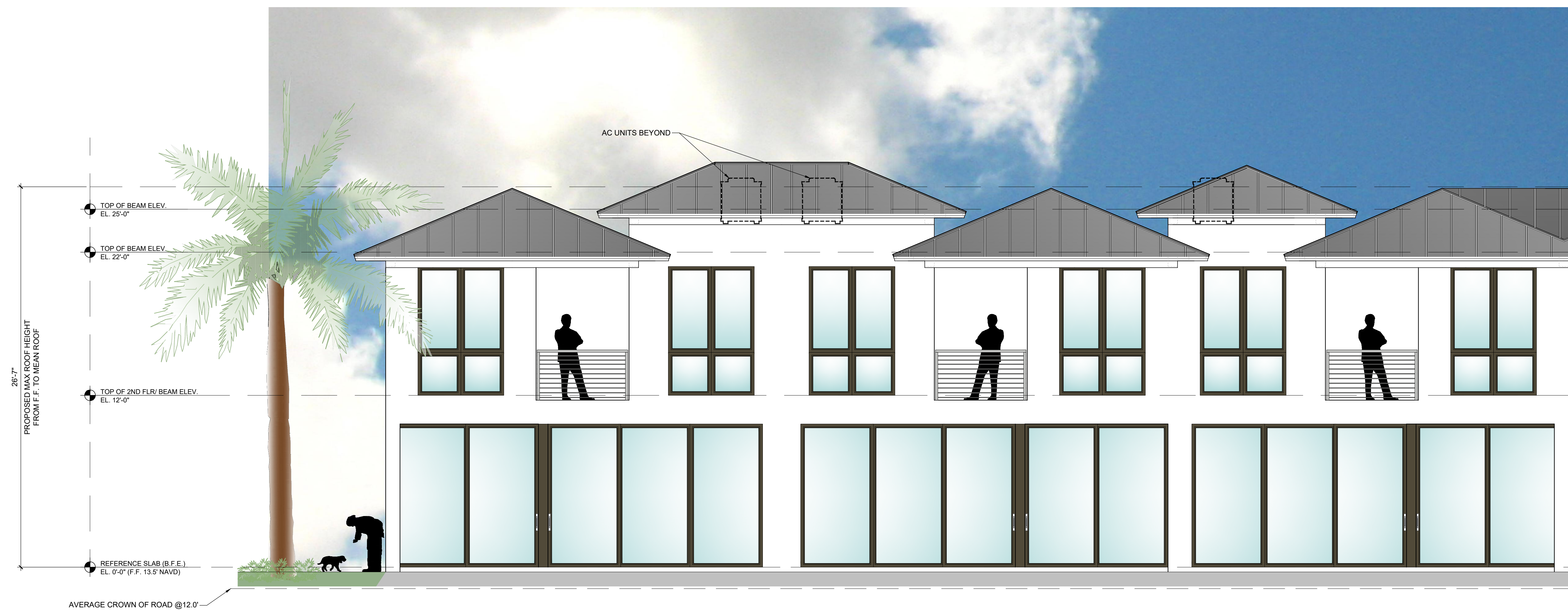
2 ENLARGED REAR ELEVATION 1/4" = 1'-0"
