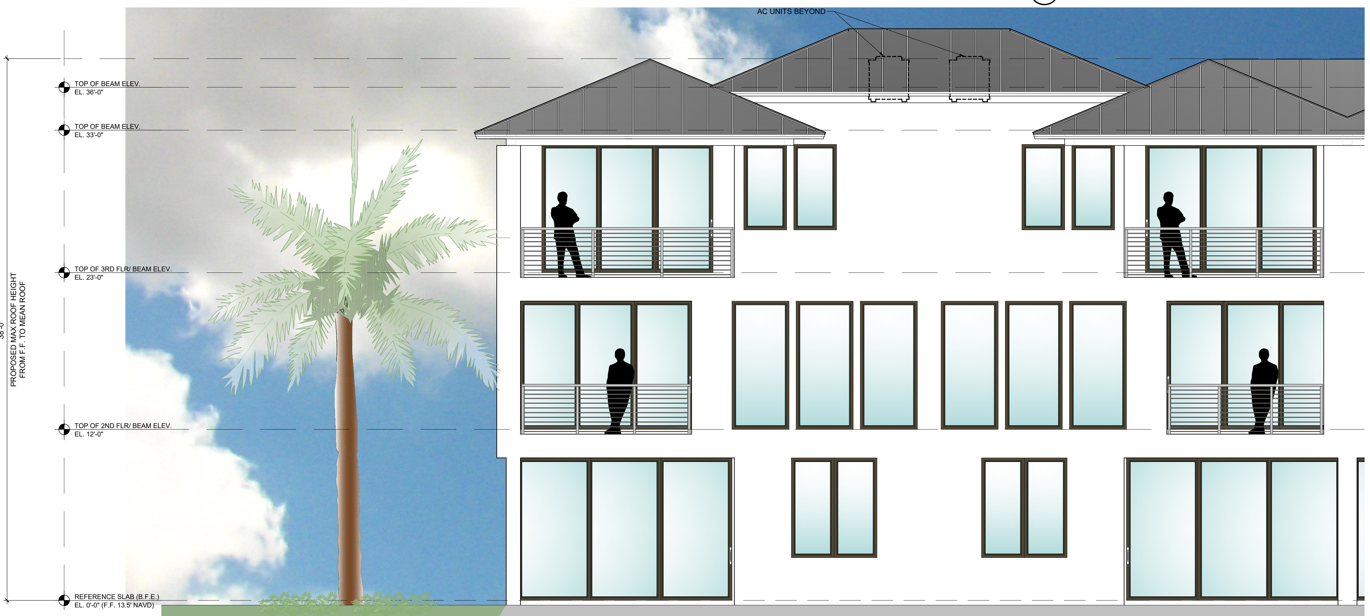
2 ENLARGED REAR ELEVATION 1/4" = 1'-0"
