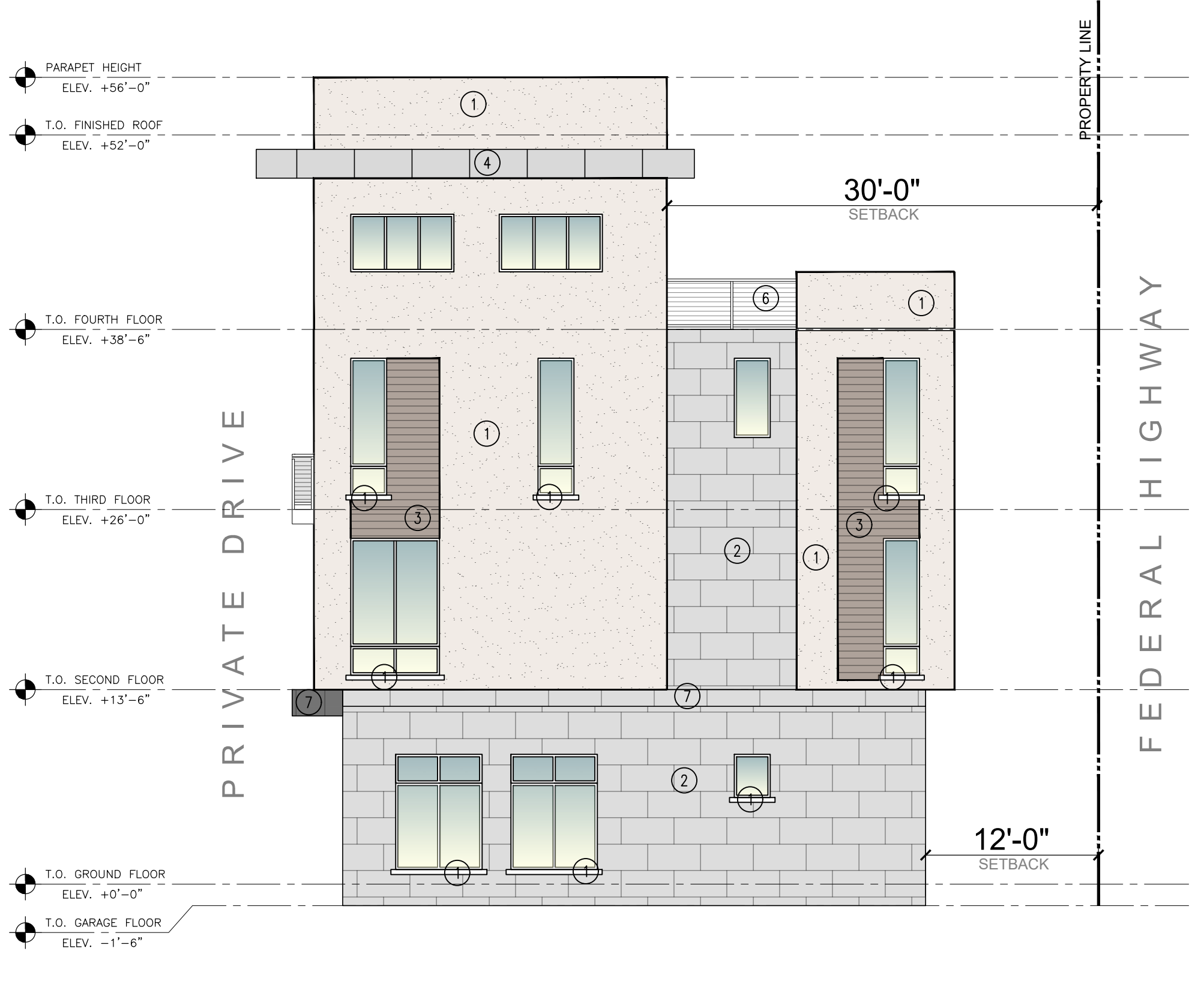
4 A.201 BUILDING 1 NORTH ELEVATION SCALE: 1/8" = 1'-0"
