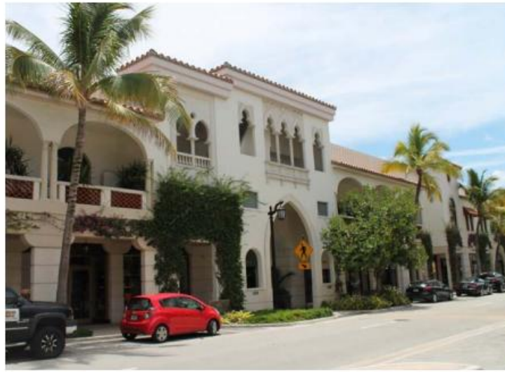
150 WORTH AVENUE PALM BEACH, FL. This mixed use commercial building has a multi-leveled parking garage integrated into its design; however, the variation of heights and the use of arcades and loggias and an interior courtyard help break down the mass and make the building compatible in scale with the surrounding context.
