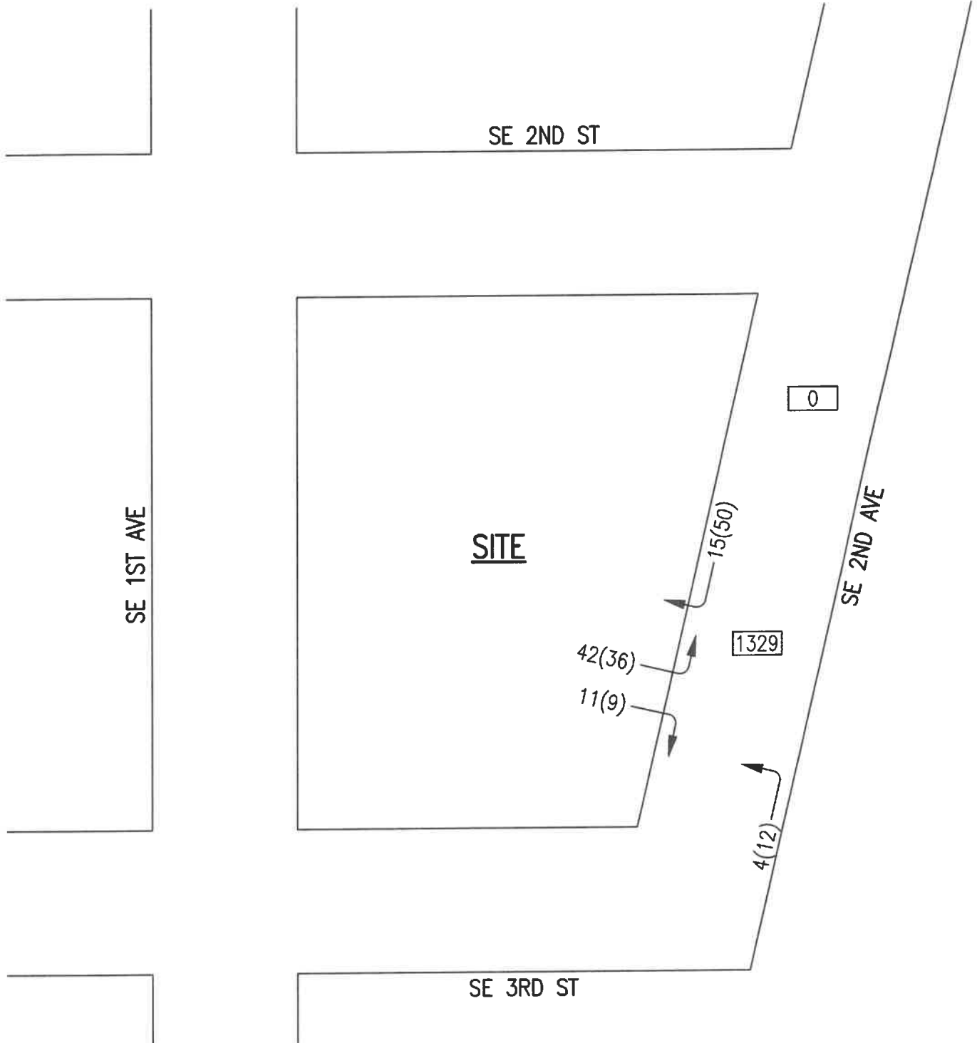
FIGURE 2 PROJECT TURNING MOVEMENTS
