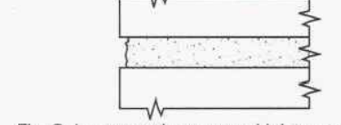
Fig. 2. Improperly prepared joint — too shallow.
