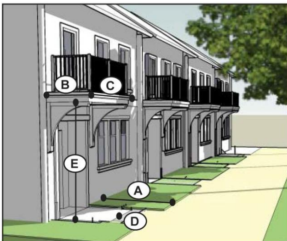
Figure 4.4.13-19 Bracketed Balcony Frontage Type
