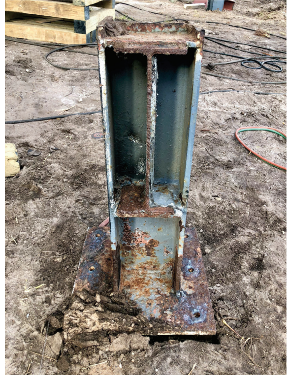
CORRODED STEEL COLUMN AND PLATE REMOVED MARCH 11, 2020
