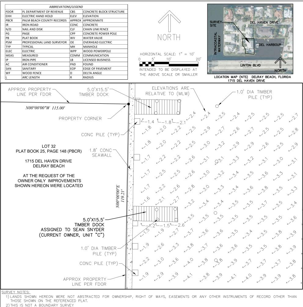
3) ELEVATIONS SHOWN HEREON ARE RELATIVE MEAN LOW WATER (MLW) AND RELATIVE TO FLORIDA DEPARTMENT OF ENVIRONMENTAL PROTECTION TIDE INTERPOLATION POINT #54 (-2.15')
