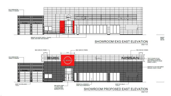
Existing (Top) and Proposed (Bottom) Front East Elevation
