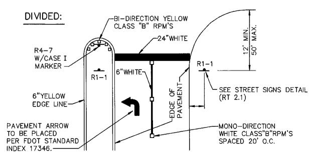
NOTE: ALL STRIPING AND DELINEATION TO CONFORM TO THE REQUIREMENTS OF THE MANUAL ON UNIFORM TRAFFIC CONTROL DEVICES, (MUTCD) LATEST ED.
