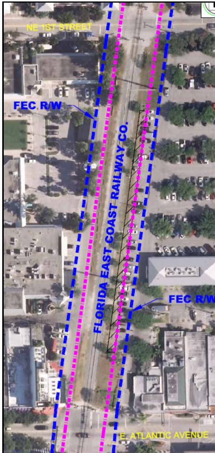
Figure 9 - New Railroad Enhancement Impacting Existing Parking Spaces
