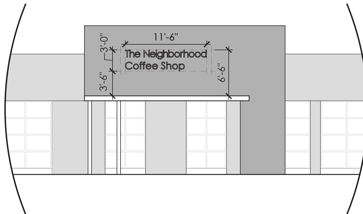
Enlarged West Elevation (Tenant Name for Example Only) Scale 1/8" = 1'-0"
