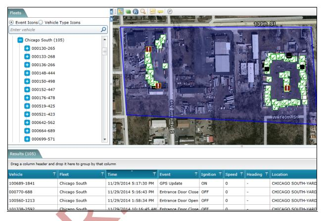
To display the location of all vehicles in a specific fleet, left click on the fleet name. The vehicles will be located and displayed on the map and included in the text list at the bottom of the map.
