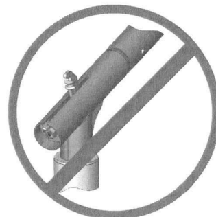
Slot in rafter allows water corrosion
