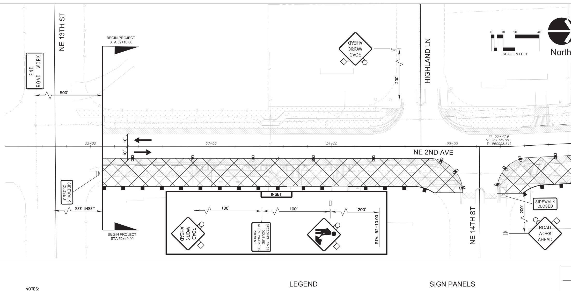
1.ALL STRIPING AND DELINEATION TO CONFORM TO THE REQUIREMENTS OF THE MANUAL ON UNIFORM TRAFFIC CONTROL DEVICES, (MUTCD) LATEST EDITION. 2.ALL CROSSWALK SIGNS AND ADVANCED PAVEMENT MESSAGES TO BE DESIGNED AND INSTALLED PER FDOT STANDARD (INDEX NO. 17346). 3.SEE LANDSCAPE PLANS FOR REMOVAL/RELOCATION OF TREES, SHRUBS, AND ALL
