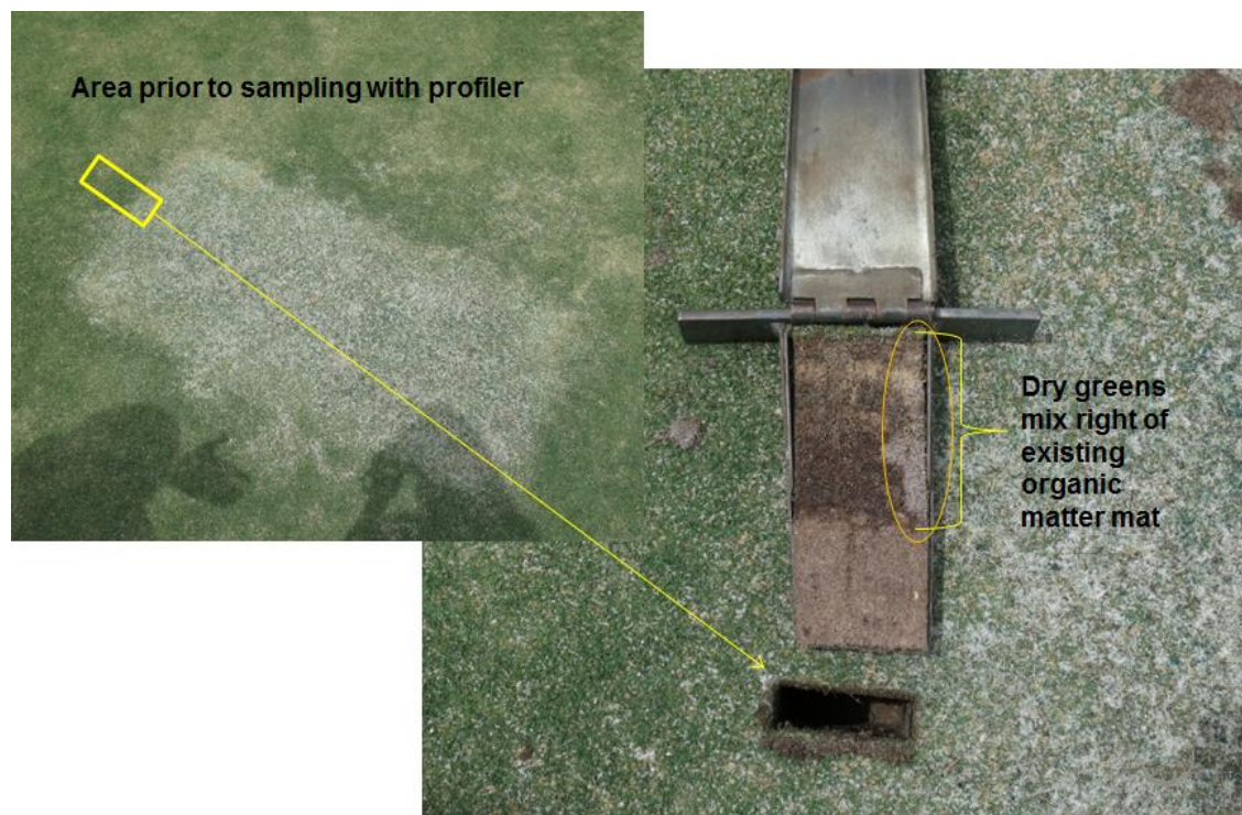
Picture 2: Comparison of soil properties of dying square of previously laid sod (right portion of profile) adjacent to existing soil
