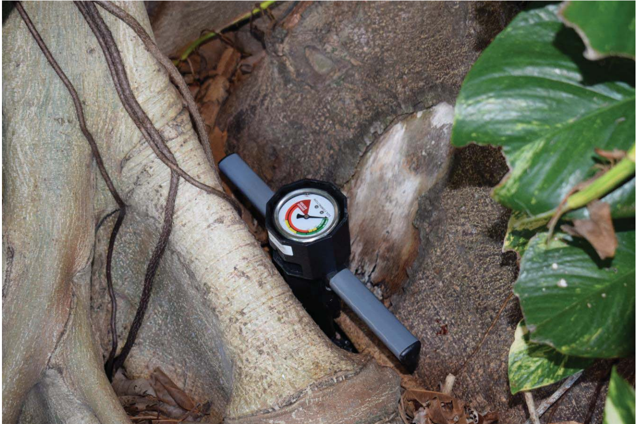
Soil penetrometer used to measure depth of cavity. No living wood tissue found beneath stem on both north and south sides.
