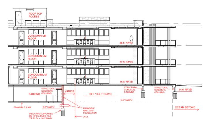
The structure is supported on 18 inch diameter concrete piles with pile caps, the piles extend to a tip elevation of -30 feet NAVD. The depth of scour anticipated at the single piles is 3 feet and the depth of scour below pile caps is anticipated to be 5 feet.
