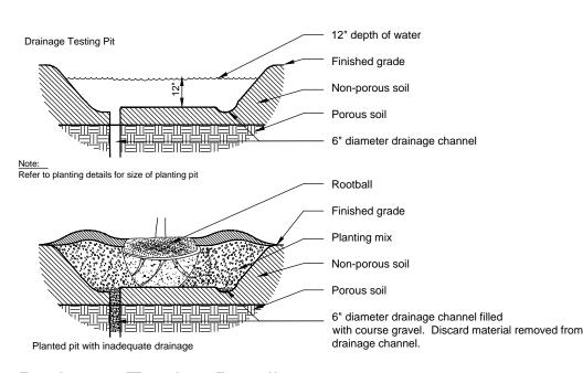
Drainage Testing Detail
