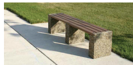
LOBBY BENCH Manufacturer: Doty & Sons Item No. 54651, 72" Detail: 72", 402lbs Concrete legs to have SB6 finish (sandblast) Seat to be 4 boards recycled plastic lumber (color is Gray RPL3) Mount to concrete pads with anchor kits item no. AK1010 (2 per lobby bench)
