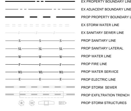
EX PROPERTY BOUNDARY LINES — – – — EX ADJACENT BOUNDARY LINES PROP PROPERTY BOUNDARY LINES EX STORM WATER LINE EX SANITARY SEWER LINE —S——— PROP SANITARY LINE -WI- PROP WATER SERVICE PROP STORM STRUCTURES
