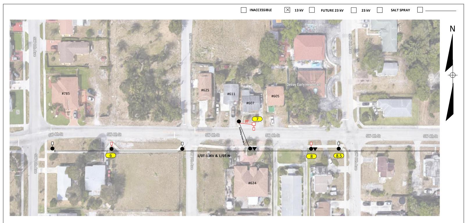
Loc.6 and 8: Install 1 AEL 40W LED ATBS 4770 Lumens on existing distribution wood pole (pending bracket length). Loc.7: Install 1 AEL 40W LED ATBS 4770 Lumens on NEW concrete pole (pending pole high and bracket length). Loc. 8.5: Remove existing light and bracket on distribution wood pole.
