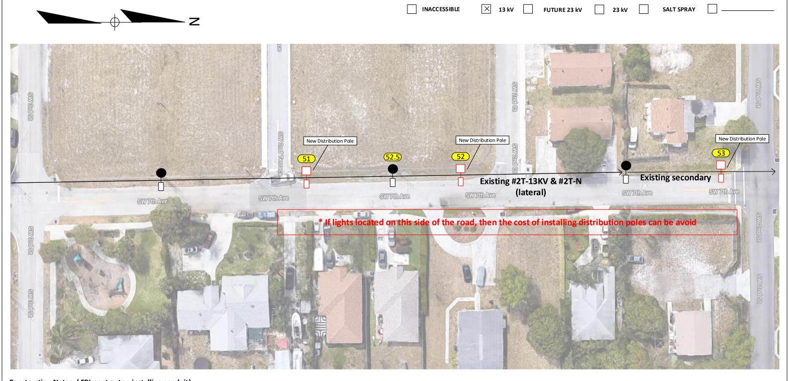
Loc. 51-53: Install 1 AEL 40W LED ATBS 4770 Lumens on NEW Distribution concrete pole (pending pole high and bracket length).
