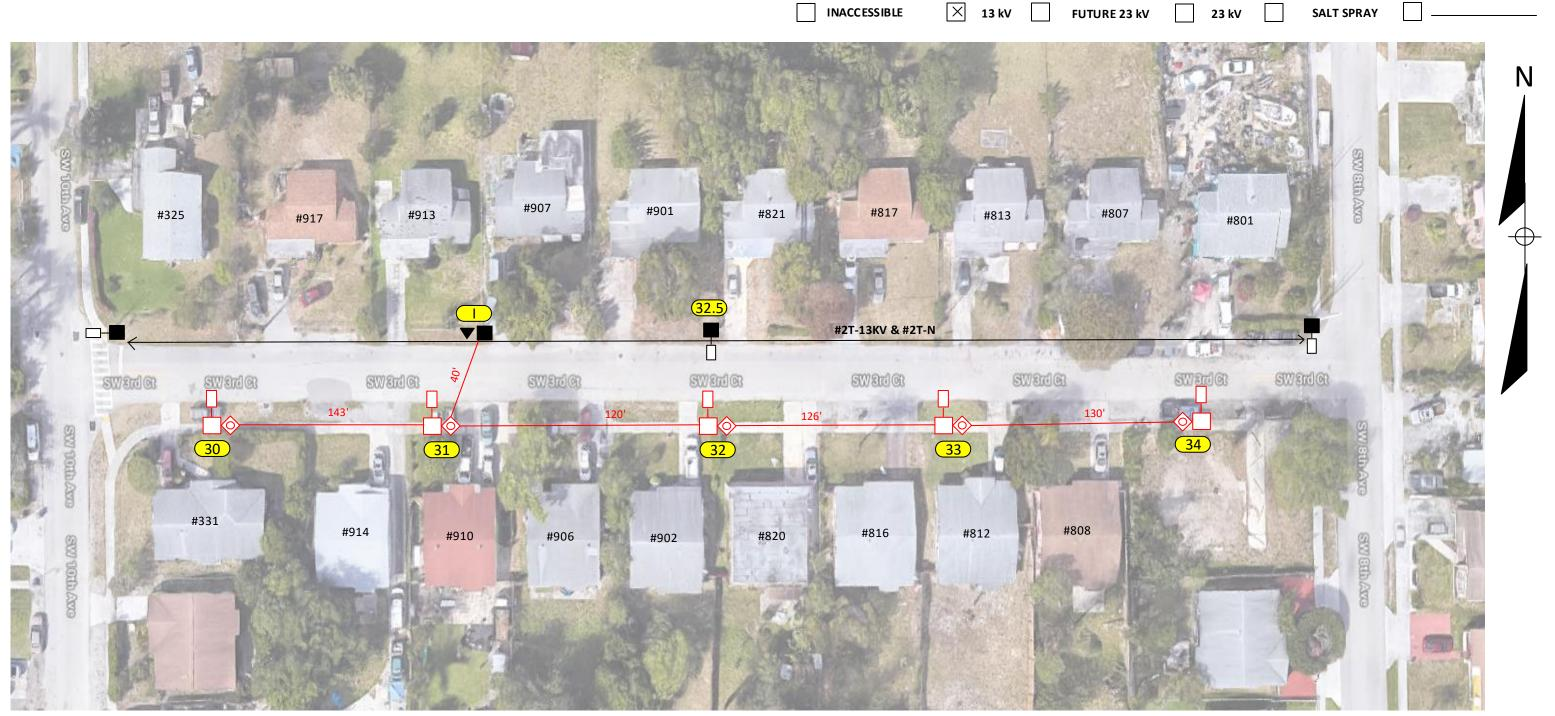
Loc. 30-34: Install 1 AEL 40W LED ATBS 4770 Lumens on NEW concrete pole(pending pole high and bracket length).
