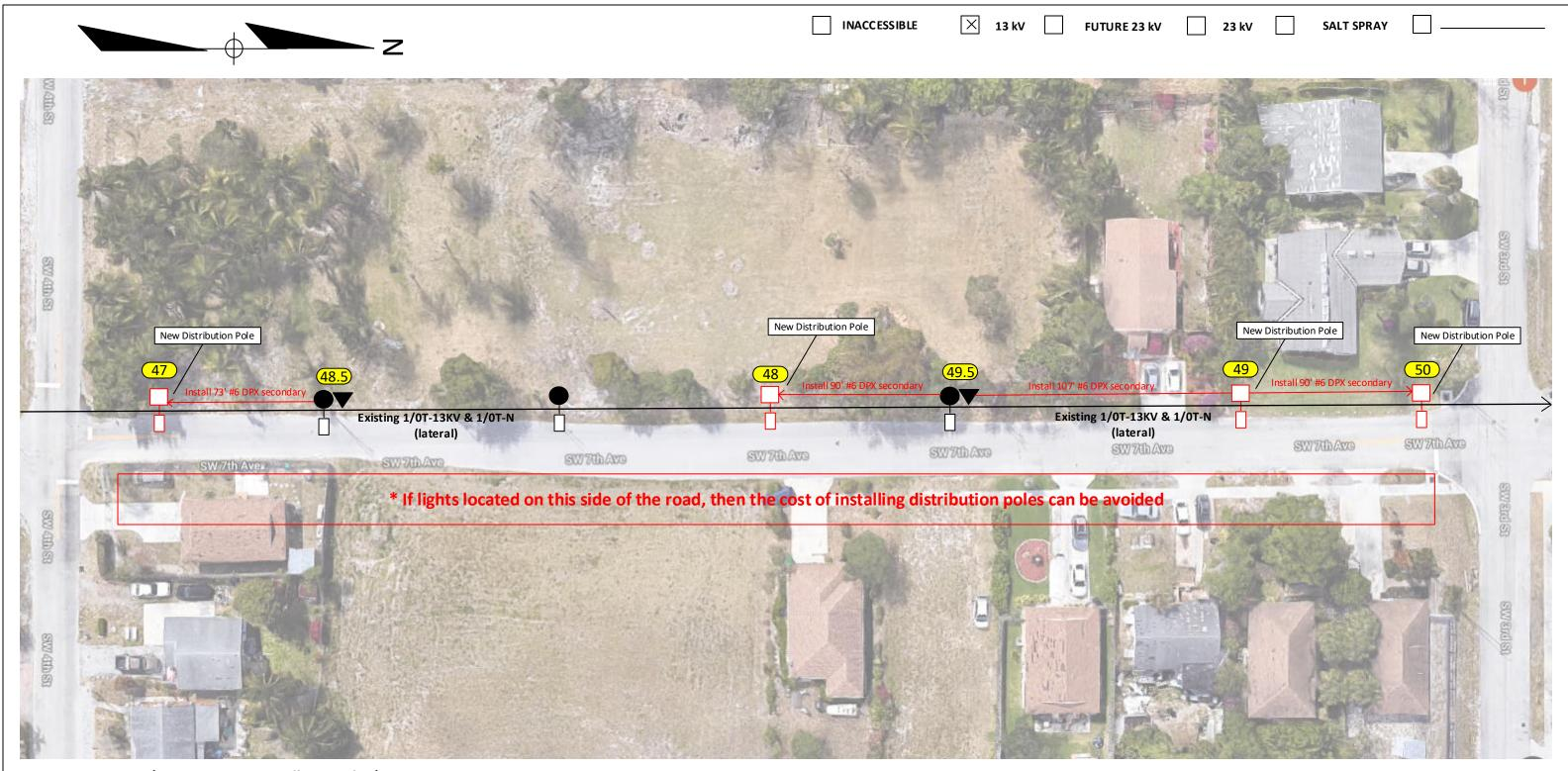
Loc. 47-50: Install 1 AEL 40W LED ATBS 4770 Lumens on NEW Distribution concrete pole (pending pole high and bracket length).
