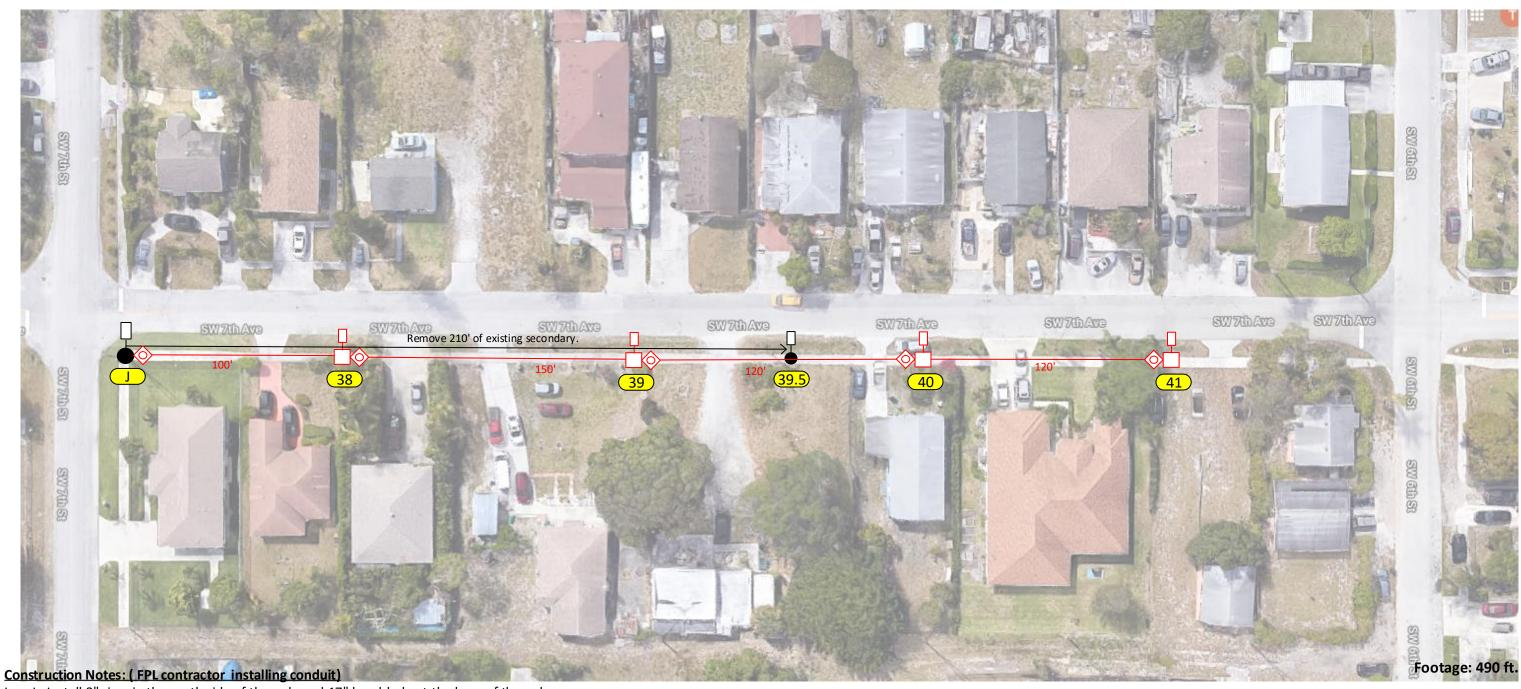
Loc. J: Install 2" riser in the north side of the pole and 17" hand-hole at the base of the pole.
