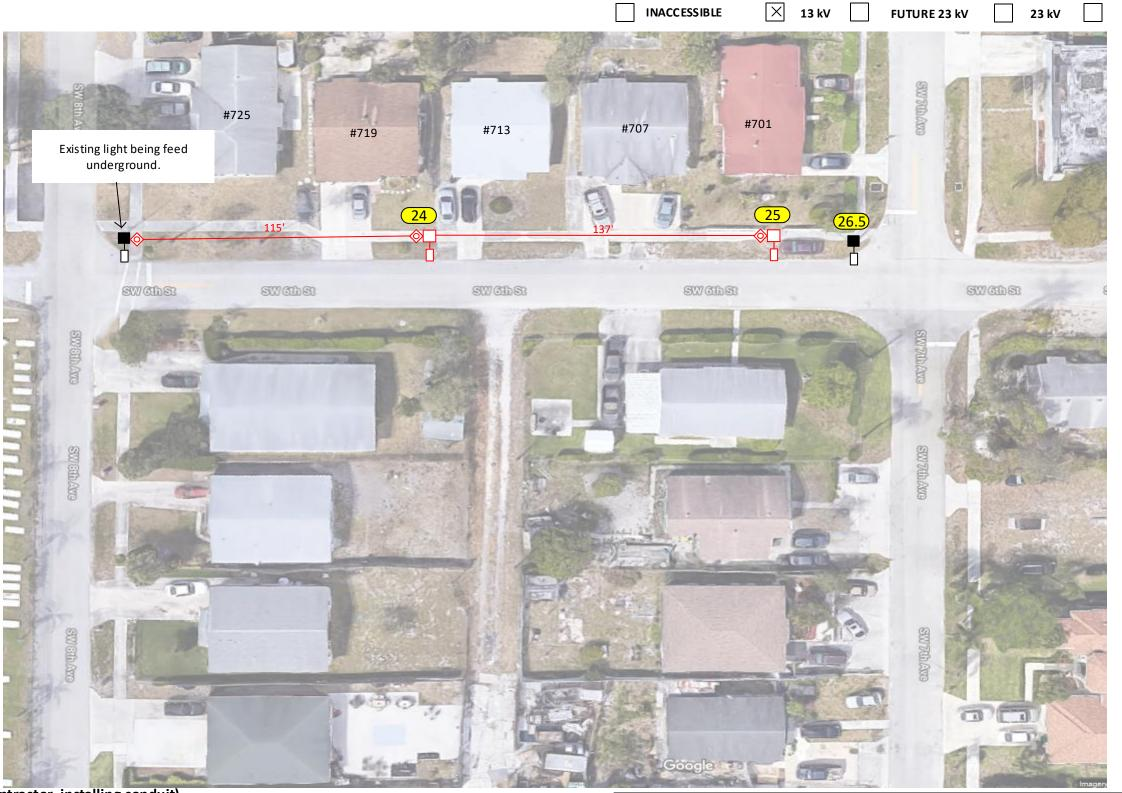
Loc. 24-25: Install 1 AEL 40W LED ATBS 4770 Lumens on NEW concrete pole(pending pole high and bracket length). Loc. 26.5: Remove street light, bracket and SL concrete pole.
