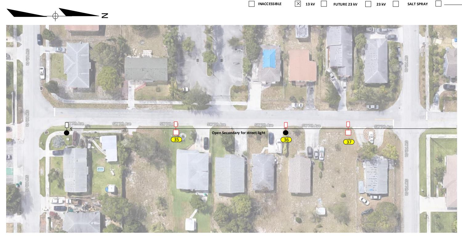
Loc. 36: Install 1 AEL 40W LED ATBS 4770 Lumens on existing wood pole (pending bracket length).
