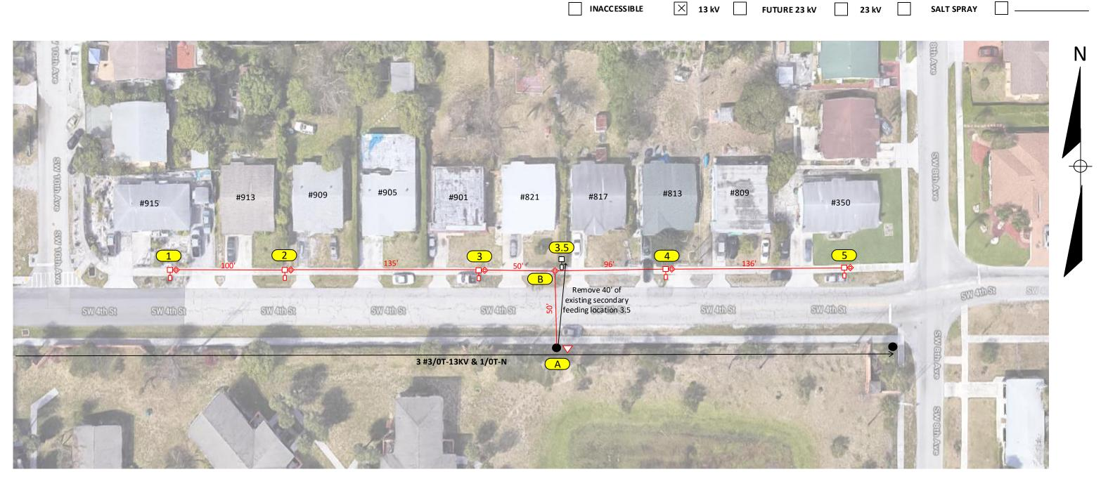
Loc. 1-5: Install 1 AEL 40W LED ATBS 4770 Lumens on NEW concrete pole (pending pole high and bracket length).
