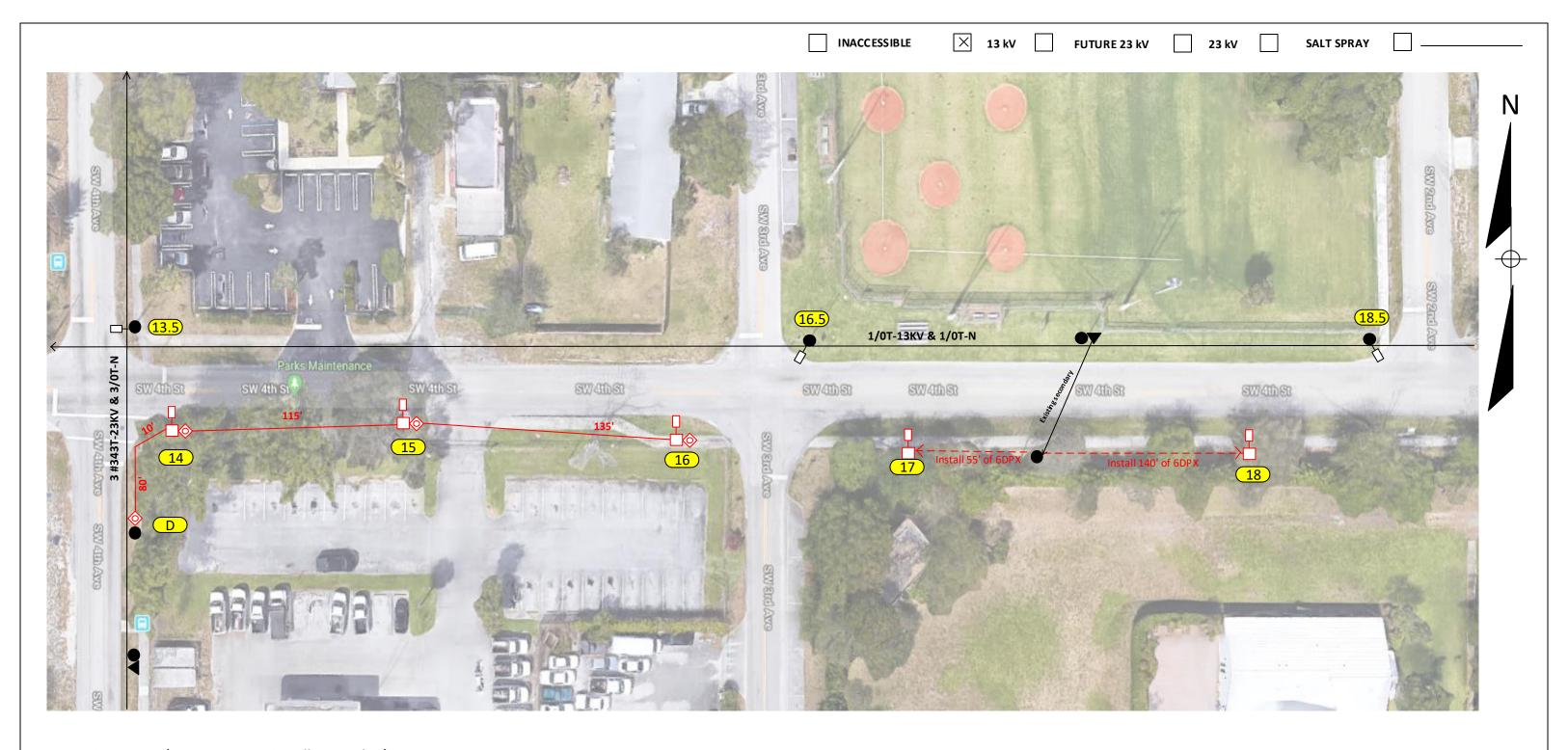
Loc. 14-18: Install 1 AEL 40W LED ATBS 4770 Lumens on NEW concrete pole(pending pole high and bracket length).
