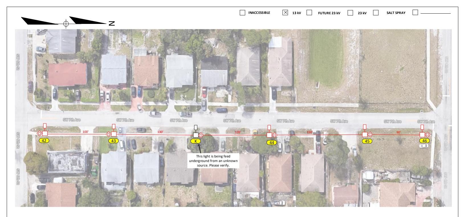
Loc. 42-46: Install 1 AEL 40W LED ATBS 4770 Lumens on NEW concrete pole (pending pole high and bracket length). Loc. K: Install 17" hand-hole. Light is being feed underground.
