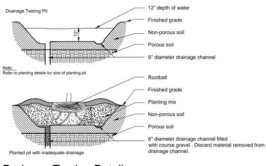
Drainage Testing Detai Not to Scale
