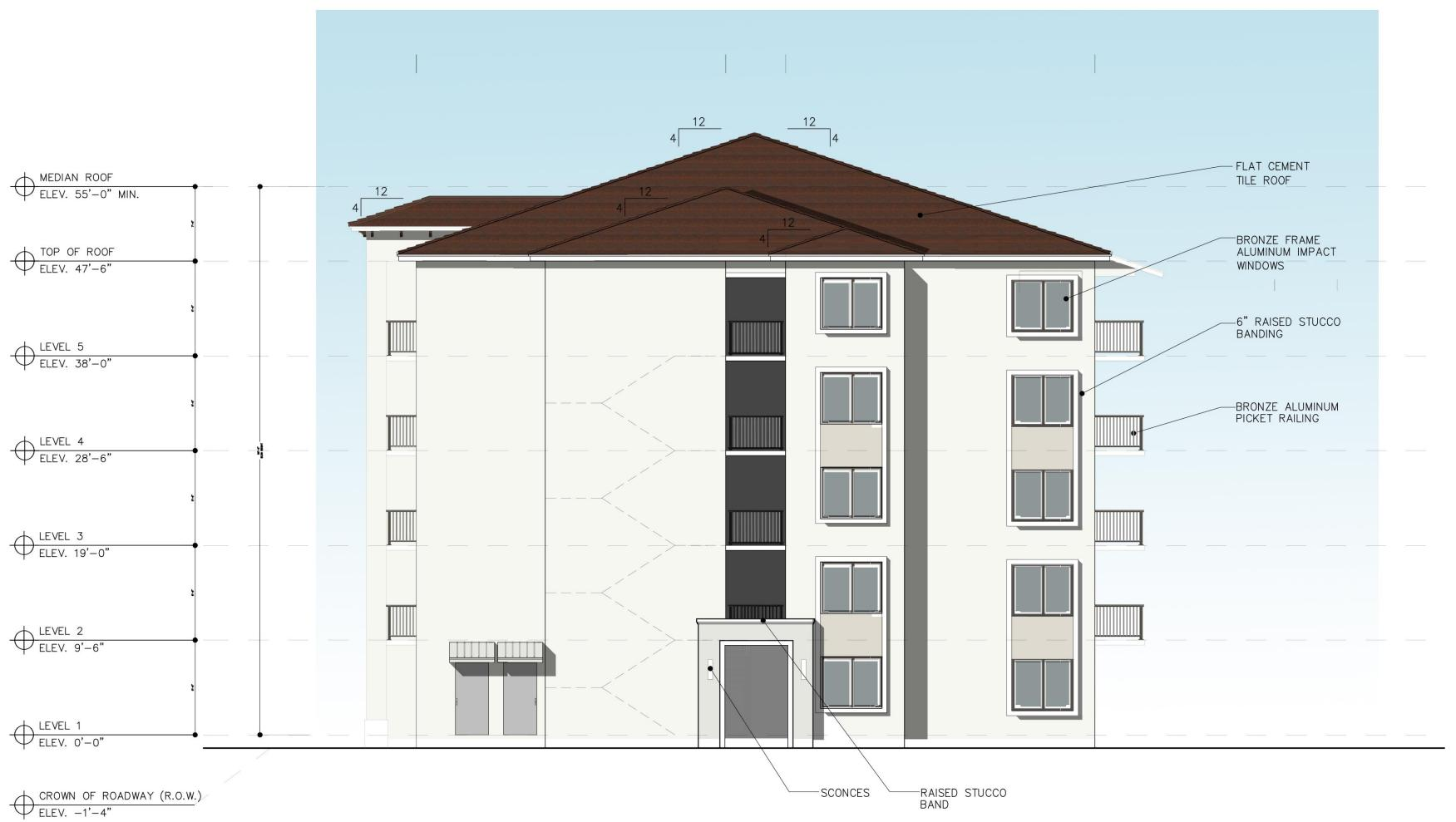
4 —RAISED STUCCO BAND BUILDING TYPE V ELEVATION SCALE: 1/8"=1'-0" 4 RIGHT
