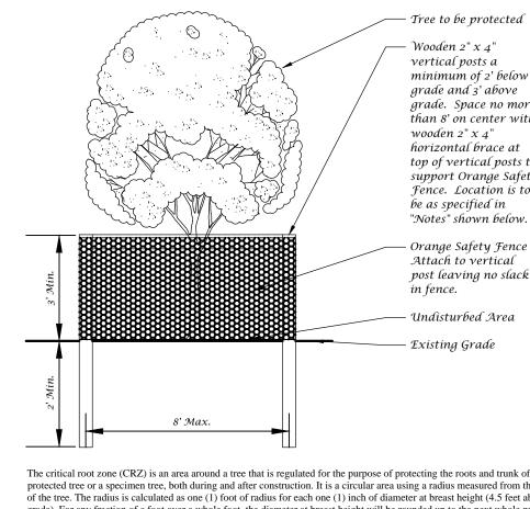
mínímum of 2' below grade and 3' above grade. Space no more than 8' on center wíth horízontal brace at top of vertical posts to support Orange Safety Fence. Location is to "Notes" shown below.
