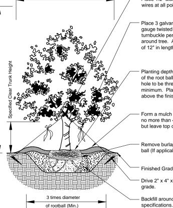
Place 1/2" diameter black rubber hose on all guy wires at all points of contact with tree.
