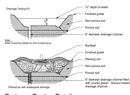
Drainage Testing Detail Not to Scale
