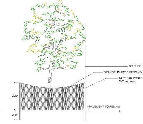
PLACE ORANGE, PLASTIC FENCING (BY TENSAR OR OTHER APPROVED EQUAL) AROUND INDIVIDUAL TREES AND TREE CLUMPS TO REMAIN ON SITE IN ANY AREAS WITHIN THE LIMITS OF CONSTRUCTION. BARRIER SHALL BE PLACED AT THE EDGE OF THE DRIPLINE OF THE THE TREE CANOPY OR AS FAR FROM THE TREE AS POSSIBLE WHERE THE CANOPY OVERHANGS PAVEMENT THAT IS TO REMAIN. BARRIER SHALL BE MAINTAINED IN AN UPRIGHT POSITION AT ALL TIMES
