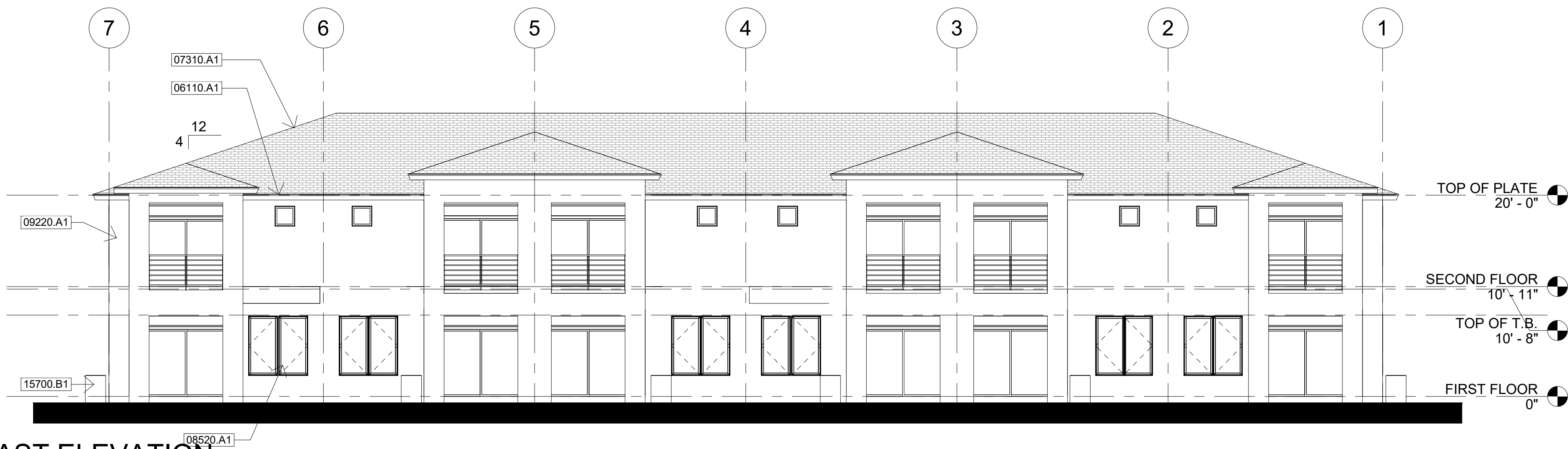
4 BUILDING EAST ELEVATION 1/8" = 1'-0"
