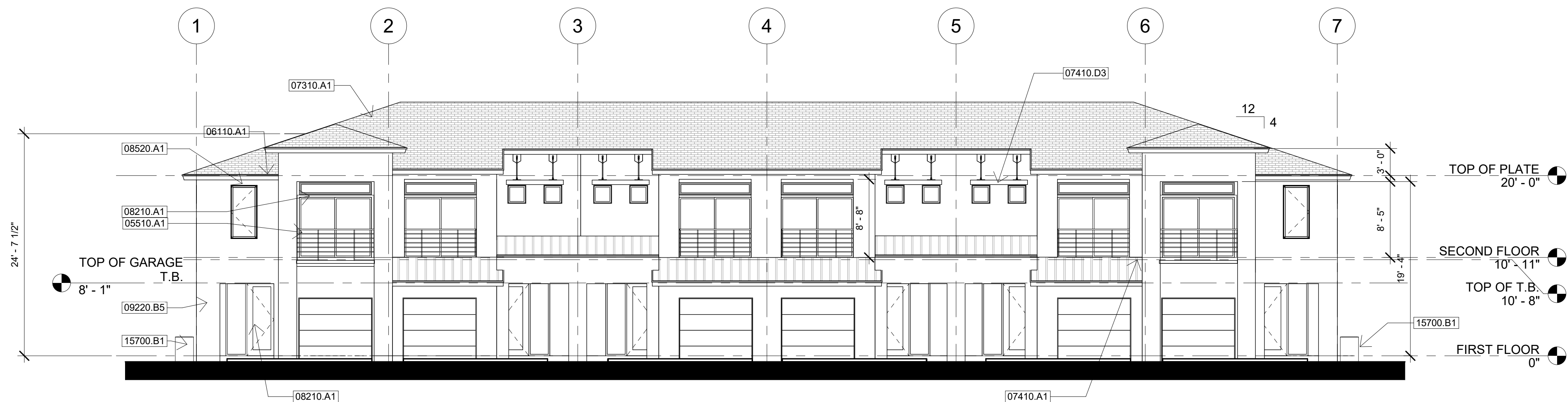
1 BUILDING WEST ELEVATION 1/8" = 1'-0"
