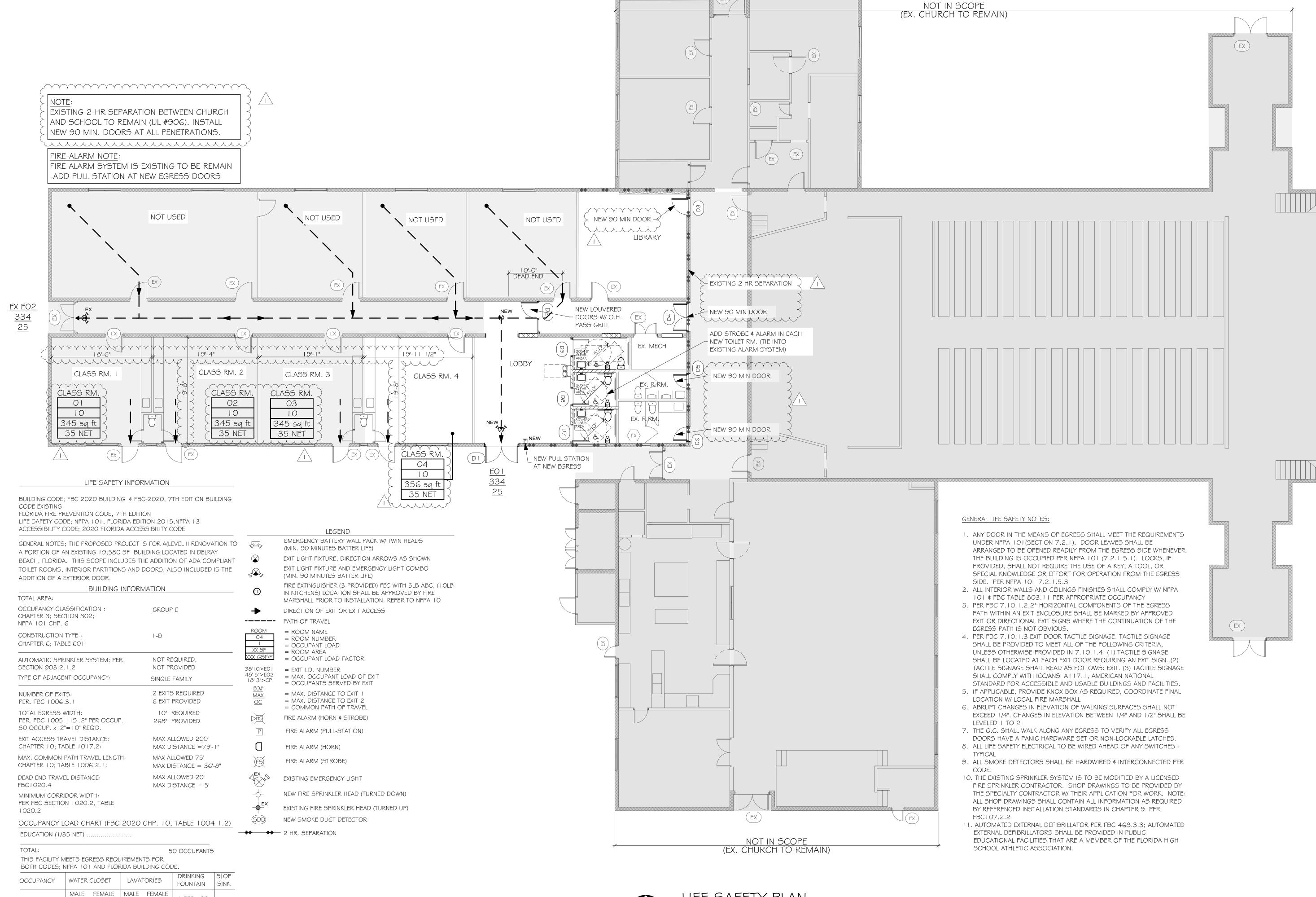
PROVIDED: 2 ΕX \*NOTE: I. FOR MERCANTILE OCCUPANCIES W/ AN OCCUPANT LOAD OF 15 OR LESS, SERVICE SINK SHALL NOT BE REQUIRED. PER FBC TABLE 403.1 e 2. DRINKING FOUNTAINS SHALL NOT BE REQUIRED FOR AN OCCUPANT LOAD OF 15 OR FEWER. PER FBC 410.2
